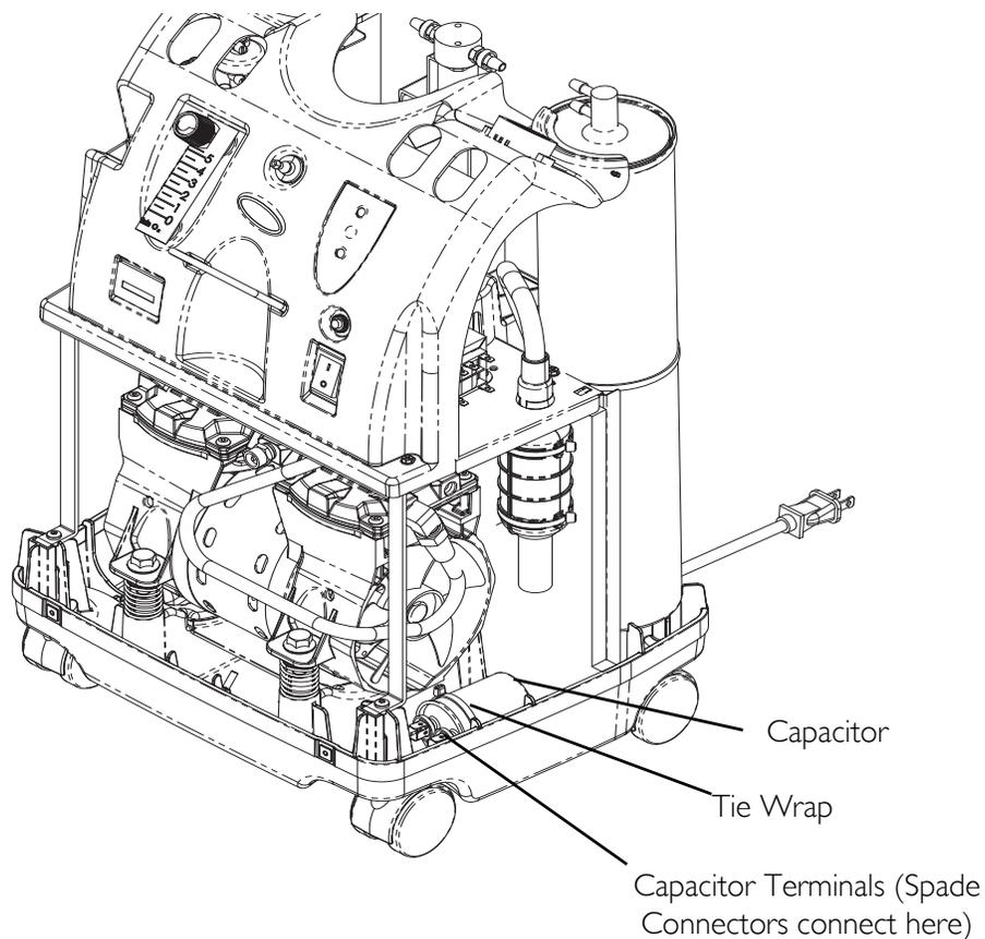
**FIGURE 7.2** Replacing Capacitor
