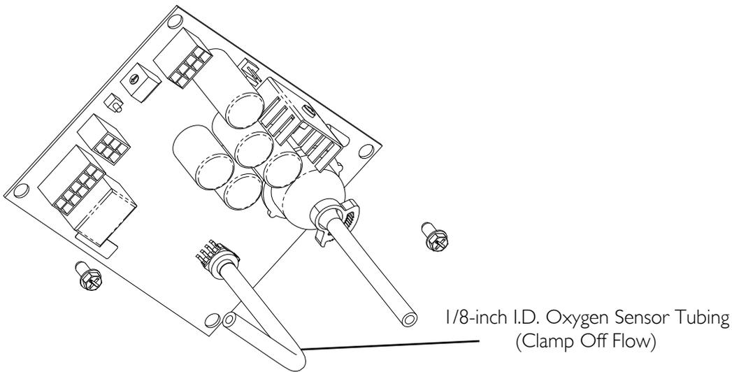
**FIGURE 24.3** Oxygen Sensor
