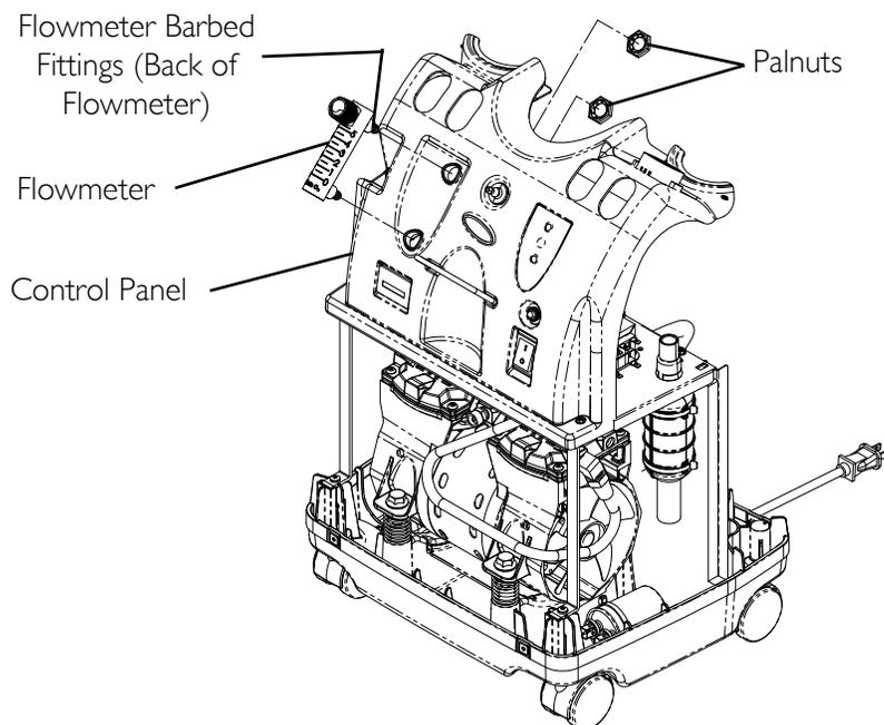
**FIGURE 18.1** Replacing Flowmeter
