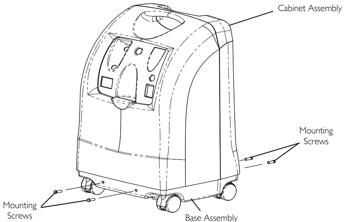
**FIGURE 5.1** Removing Cabinet
