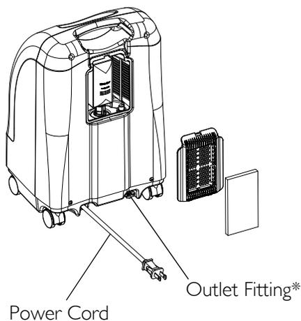
*\*NOTE: This outlet fitting is to be used only for filling oxygen cylinders with the HomeFill home oxygen compressor. The outlet fitting does not affect concentrator performance. Refer to the HomeFill owner's manual, part number 1100873, for connection and operating instructions. When not in use, the plug provided with the concentrator should be inserted into the outlet fitting. For more information about the HomeFill, contact your Invacare dealer.*
